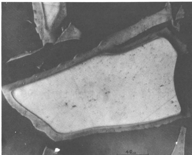
Figure 12. Particle of Duxite displaying an oxidized rim after oxidation for 3 hours at 140°C.; relief-polished surface, oil immersion, incident light; \times 378
