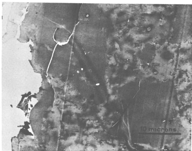
Figure 3. Dourges coke 525°C., section observed in bright field; anisotropy of grainy type; \times 1800
