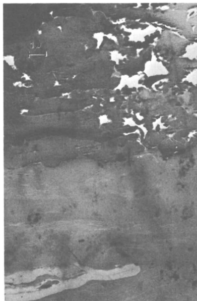
Figure 5. Contact between semifusinite (showing cellular structure) and vitrinite. This junction appeared to be transitional in the light microscope but at this magnification appears sharp. \times 4390
