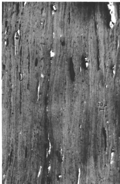
Figure 4. Light micrograph of a polished surface of a high volatile bituminous coal. The fine banding is caused by groups of sheets which cannot be resolved individually with the light microscope. \times 185
