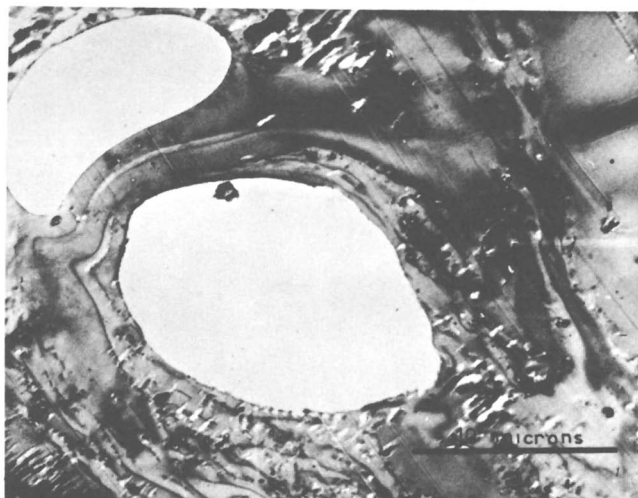
Figure 4. Drocourt coke 500°C., section observed in bright field; anisotropy of fibrous type; \times 2718
